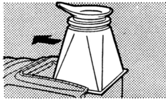
To remove the standard hood (left), first release the magazine 6 and then slide the hood backwards out of its grooved fitting. Alternative finders, such as the magnifying hood (right) can then be slid in place.
