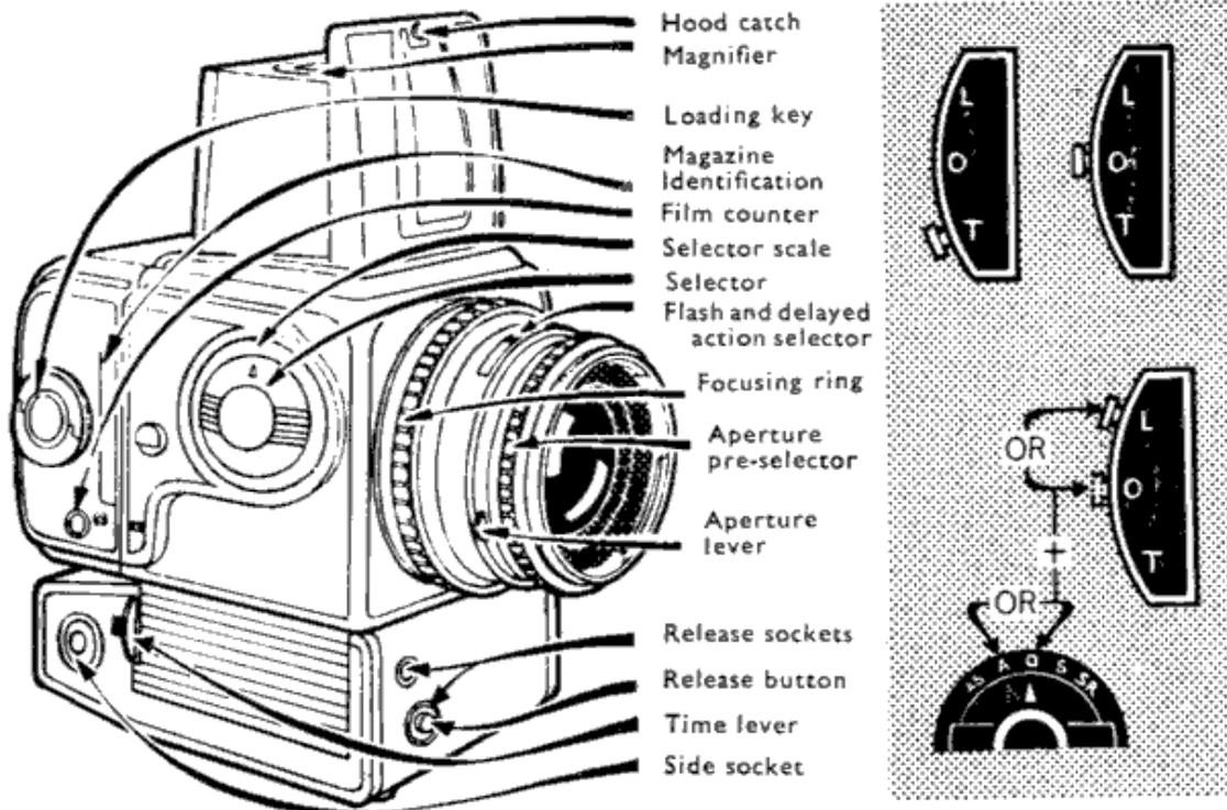
The 500EL is basically a 500C, but it has additional controls. The time lever, shown at right above, is used for exposures from 1 second to 1 minute and when making exposures with the self-timer. Moving the lever to T (with the shutter set to B) opens the shutter. Moving the lever to O closes the shutter, advances the film and re-cocks the shutter. When changing lenses, the time lever must be set to L or O and the selector scale (see below) set to A or O.
