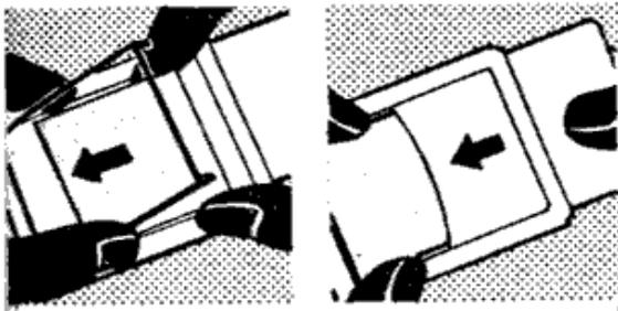
To load the cut film holder place the trimmed sheet of film below the film frame (left), fold down the latter and push in the sheath (right). This must be done in total darkness.
