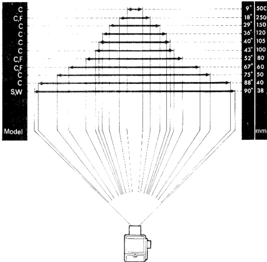
The shorter the focal length of the lens, the greater the angle of view taken in. With the interchangeable lenses the Hasselblad can thus control the angle of view - and also the scale of the image recorded.
