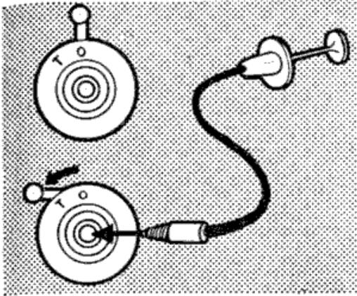
For time exposures (with the shutter set to B) the time catch on the release keeps the shutter open after pressing the release. For this purpose move the catch to the position T before releasing. Preferably make time exposures with a cable release; this screws into the release button. The shutter closes again on moving the time catch to the position O.
