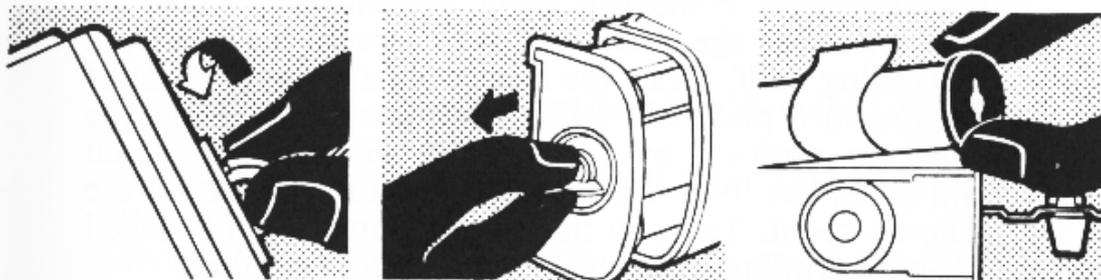
Unloading. Wind off the end of the backing paper with the loading key (left), then remove the spool holder by unlocking the spool key and withdrawing the holder (centre). Finally remove the full film spool and seal (right).
