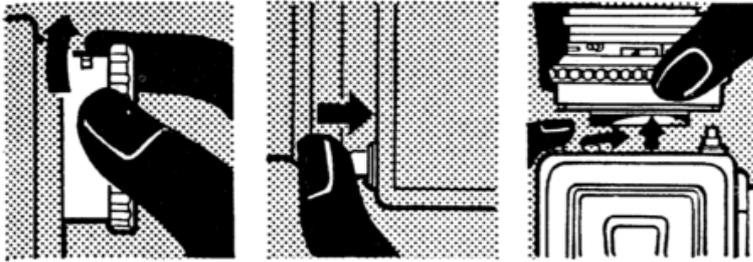
Removing the lens from the Hasselblad 500C. First tension the shutter (left), then depress the lens catch (centre), and turn the lens anti-clockwise and lift out of the camera (right).
