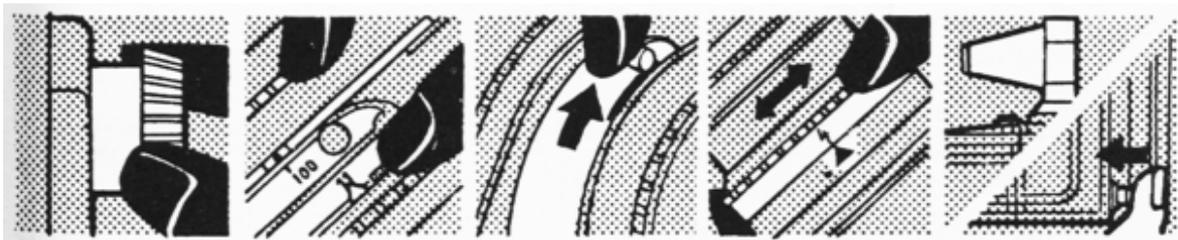
Shooting with the Super Wide. From left to right: Wind the film transport knob; set the aperture and shutter speed separately; tension the shutter; set the lens to the appropriate subject distance; view the subject through the finder and release the shutter.
