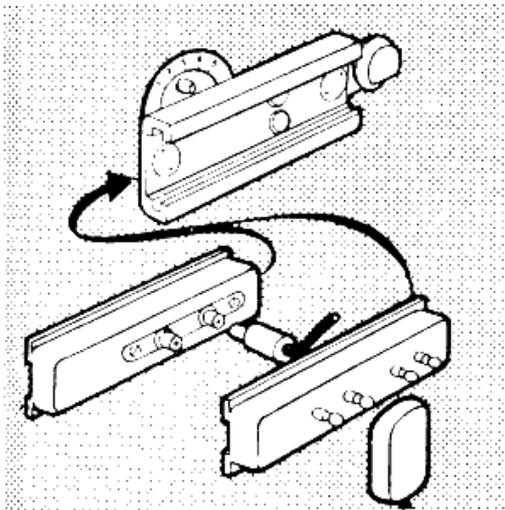
The models 1000F and 1600F have a synchronization contact built into the finder shoe at the side of the camera. The synchronization is here adjustable by moving the small control above the shoe to a series of numbers from 1 to 5. To connect the flash, a flash shoe fits into the finder shoe. The flash shoe carries either two co-axial sockets, or two pairs of two-pin sockets (older version). The outlets in each case are marked "flash" (for flash bulbs) or "strobe" (for electronic flash).
