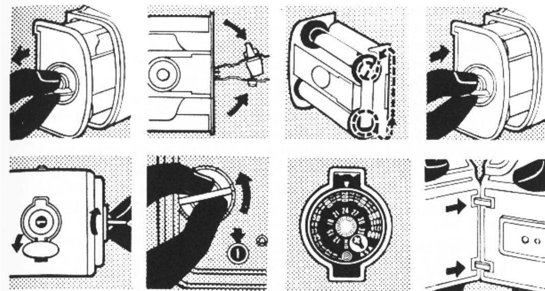
Top row: Unlock the spool holder key (left) and pull out the spool holder. Open the spool holder arms (centre left), insert the full film spool and thread the backing paper around to the empty take-up spool (centre right). Insert the loaded spool holder into the magazine and lock (right).
